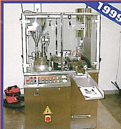
KWANG DAH AUTOMATIC CAPSULE FILLING MACHINE, MDL. KDF-6
