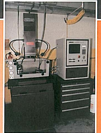
1994 HANSVEDT Foreman CNC EDM with M-Pulse 3025 Power Supply
