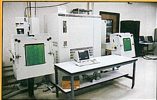
SCHLUMBERGER Sentry S90 Memory Tester, dual head
