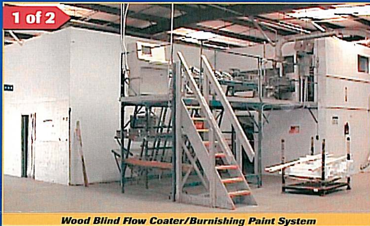
Wood Blind Flow Coater/Burnishing Paint System
